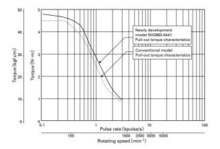
Fig. 7: Comparison of Pulse rate – Torque Characteristics for SH2863-0441/ 0411
