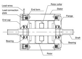
Fig. 3: Structure of the Motor
